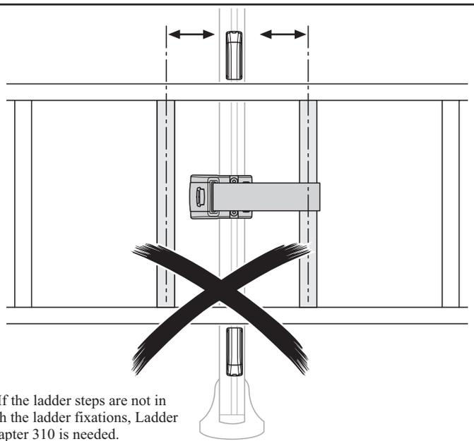
**GB** If the ladder steps are not in line with the ladder fixations, Ladder Step adapter 310 is needed.
